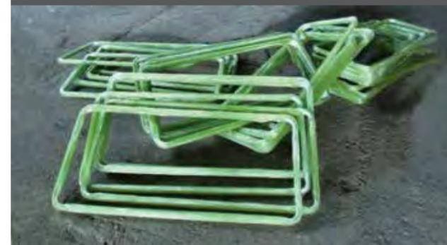
ATP has developed a new production technology for the production of the stirrup where we do not bend a straight rebar to create a stirrup, but instead directly produce the bent or closed stirrup as a final product. Closed stirrups allow better confinement of concrete and the smaller radius enables the reinforcement to be closer to the surface to increase the total mechanical characteristics of the concrete structure.
