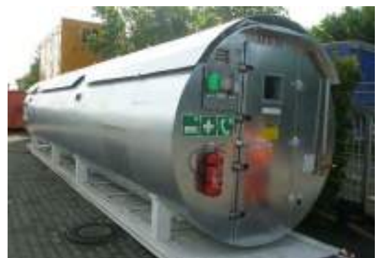
Refuge chamber for 20 people and 12hours standalone operation
