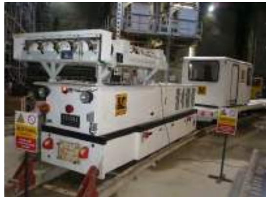
Firefighting Emergency Loco with oxygen supply for engine
